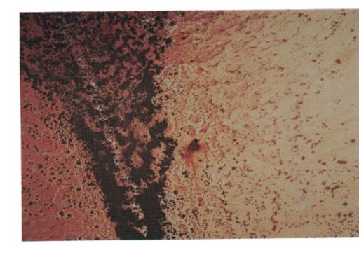
I-20 Same as Photo I-19, except the rust tubercle has been removed to examine the substrate. Note moderate to severe pitting present.
